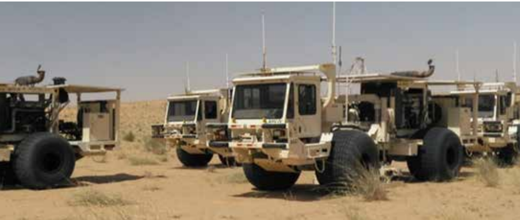
Vibrator trucks from BGP Crew 8636B on the R3 East survey area.
